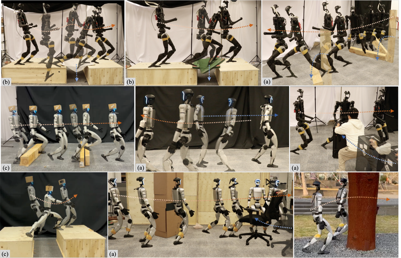
Fig. 1: Overview. VB-Com enables humanoid robots (move direction in orange arrow) to traverse dynamic terrains and obstacles (move direction in blue arrow). The perception deficiency is introduced by (a) suddenly appearing obstacles/hurdles, (b) deformable gaps, and (c) sensor occlusions. We demonstrate the effectiveness of VB-Com on both robots of Unitree G1 and H1.
